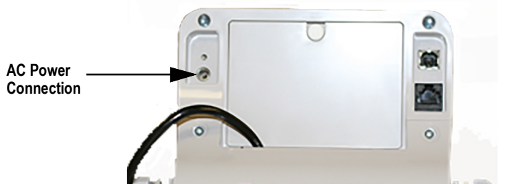
Figure 2-5. Power Connection Site
