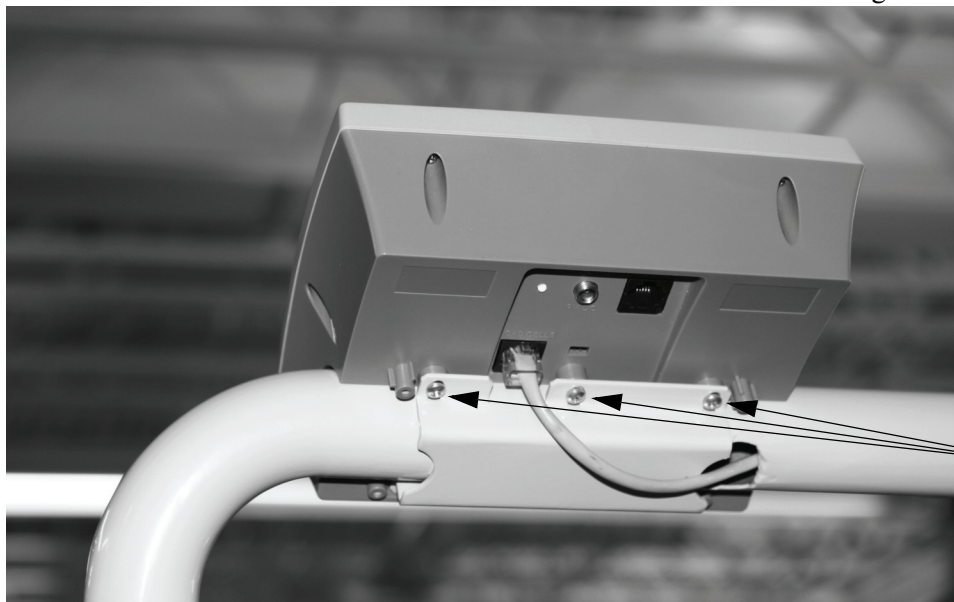
Figure 2-3. Mounting Bracket Screw Location
