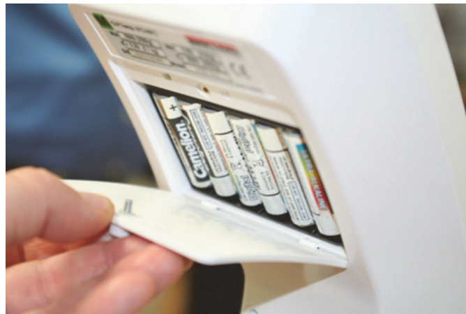
Figura 3-8. Batteries in Battery Chamber
