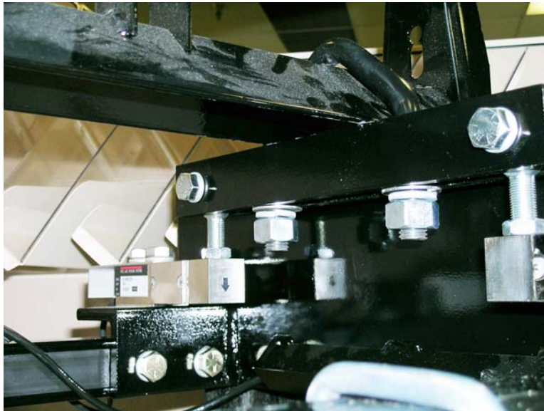
Figure 2-12. Mount Idlers to Scale Carriage Using V-Bolts
