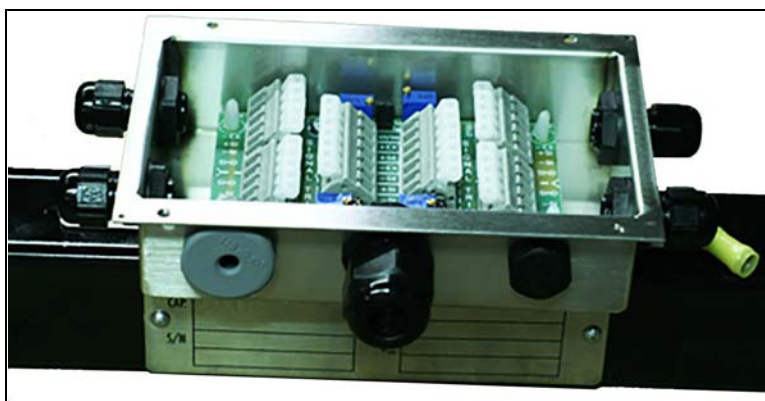
Figure 2-7. Junction Box Interior
