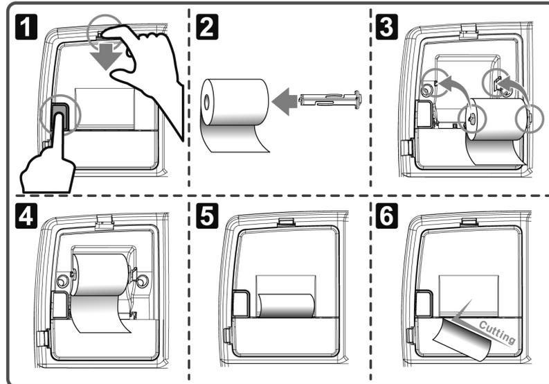
Figure 3-4. Replacing Thermal Paper in Printer Unit
