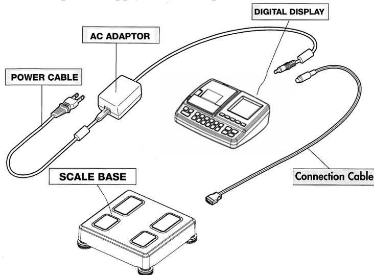
Figure 3-2. Competitor Series Component Parts
