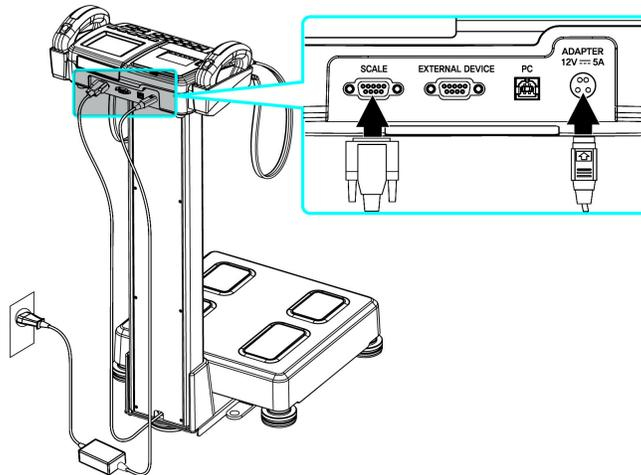
Figure 3-11. Power Supply and Scale Cable Connection Locations
