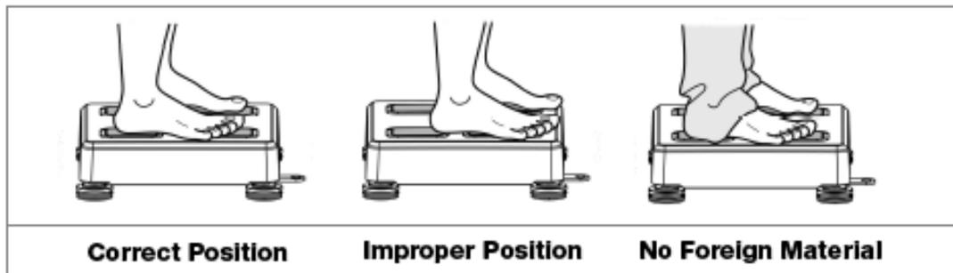
Figure 5-1. Correct Stance on Scale Base
