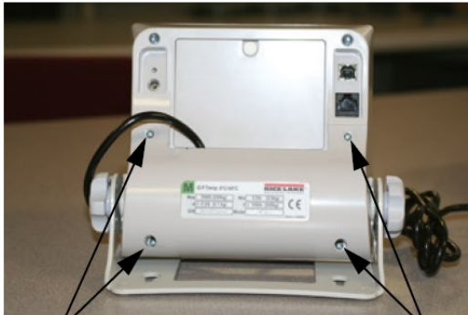
Remove four screws to access setup switch
