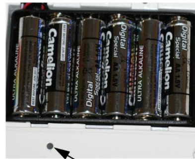
Setup switch location
