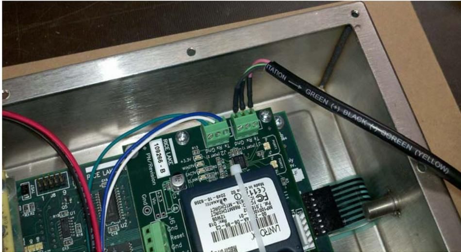
Figure 5. Connect Three Wires to Configure the Unit
