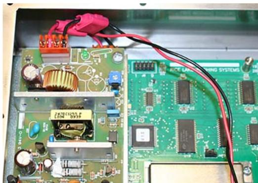
Figure 3. CLS-420 Installation Red and Black Wire Location
