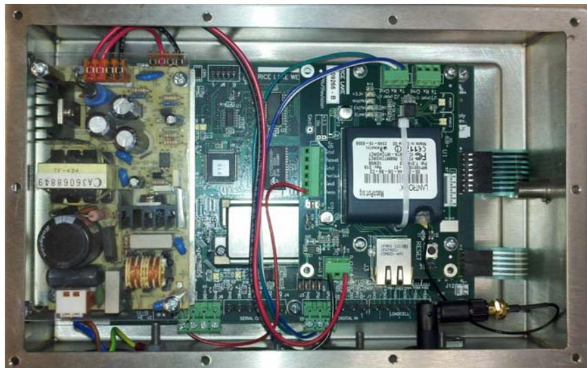
Figure 4. WLAN Option Installed in 420 Indicator
