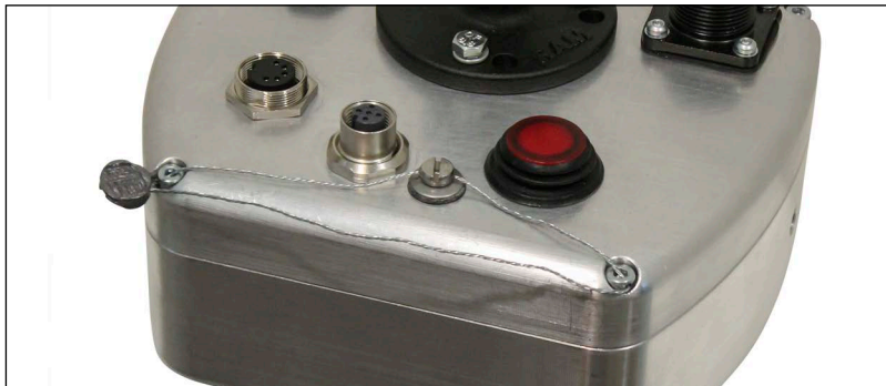
Figure 2-12. Sealing the Enclosure – No Access
