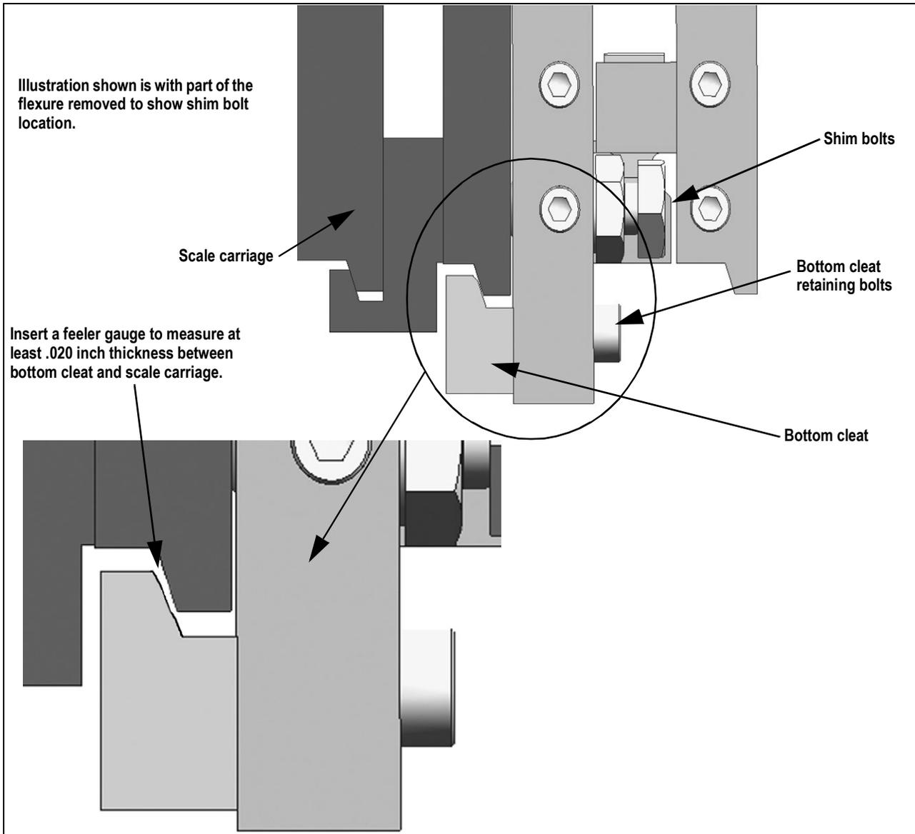
Figure 2-6. Bottom Cleat Location and Assembly
