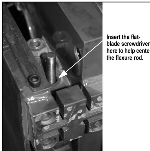
Figure 3-19. Centering the Flexure Rod
