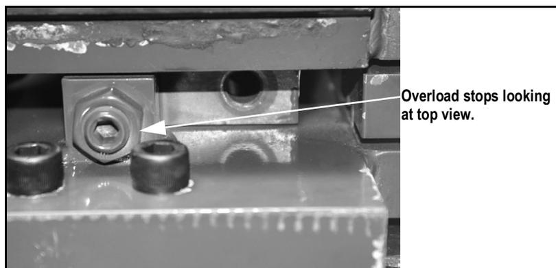
Figure 3-14. Overload Stops
