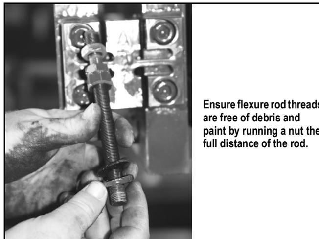
Ensure flexure rod threads are free of debris and paint by running a nut the full distance of the rod.
