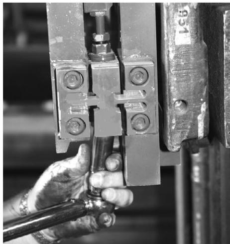
Figure 3-21. Tighten Lower Nut
