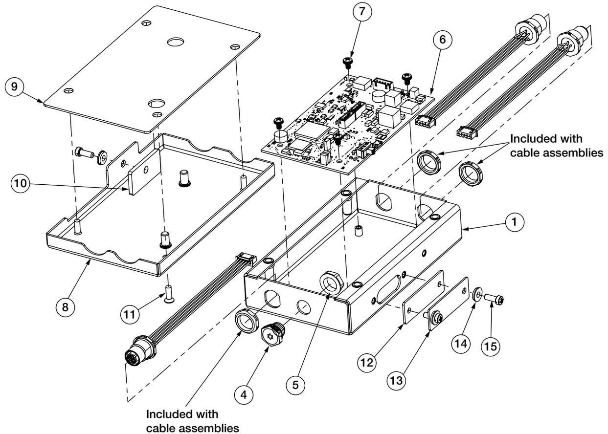
Figure 3-3. CLS-IM Junction Box Assembly (PN 191642)
