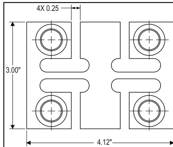
Figure 3-22. Flexure Chassis
