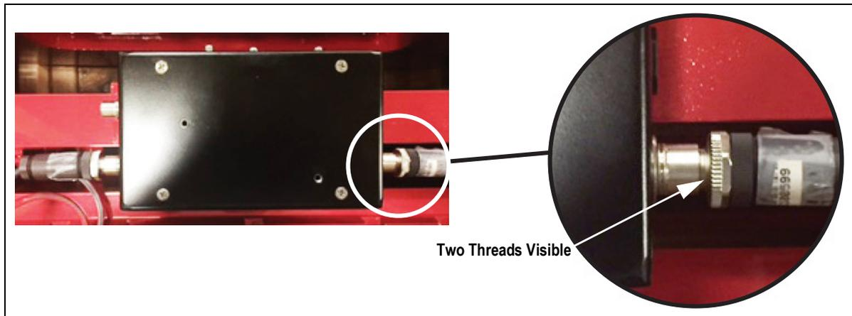
Figure 3-6. Connect Load Cell Cable to Junction Box
