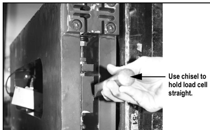
Figure 3-17. Use Chisel to Hold Load Cell Straight
