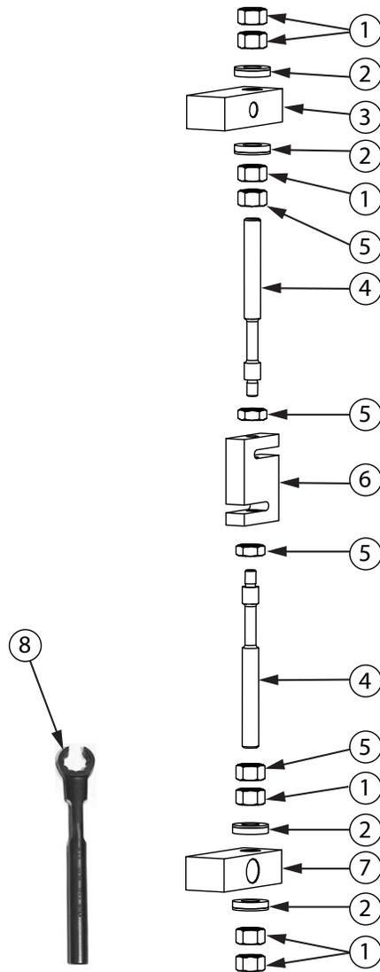
Figure 3-2. Load Cell Replacement Kit Parts Illustration
