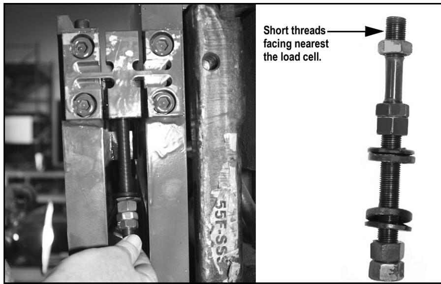
Figure 3-16. Installing Flexure
