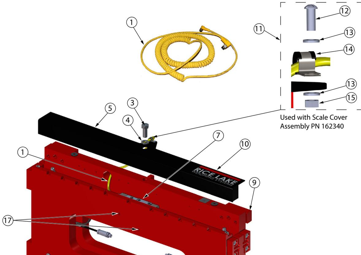
Figure 3-1. Cargo Lift Scale Assembly Parts Illustration
