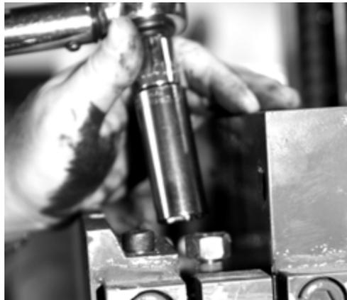
Figure 2-3. Removal of Hex Nut (Item #1 in Figure 2-2)
