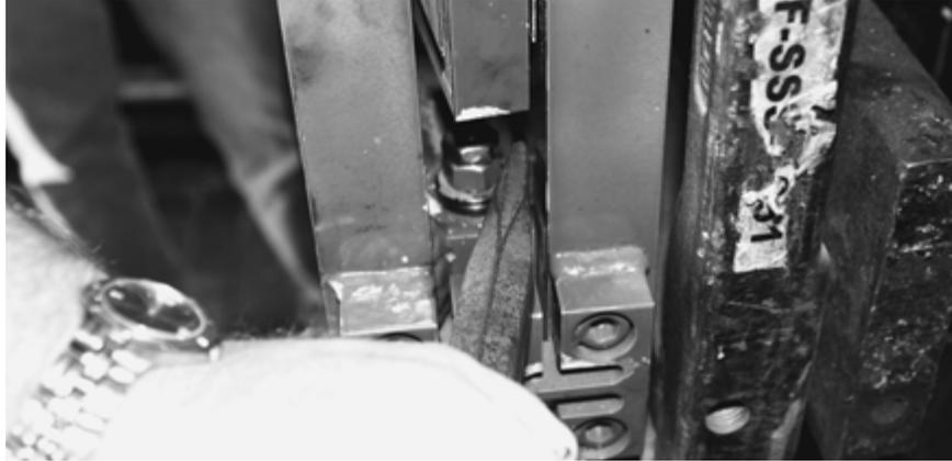
Figure 2-12. Centering the Load Cell Using a Chisel
