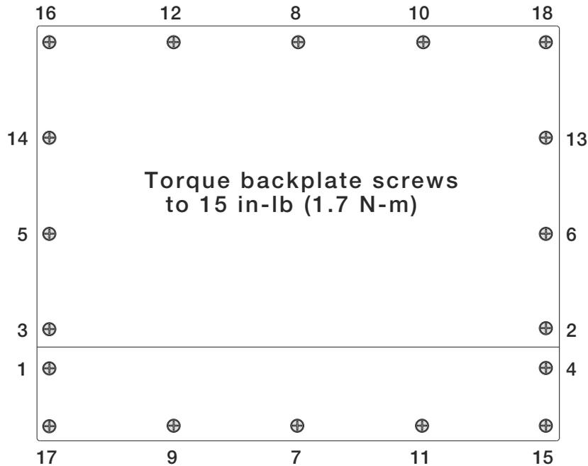
Figure 5-8. Torque Pattern
