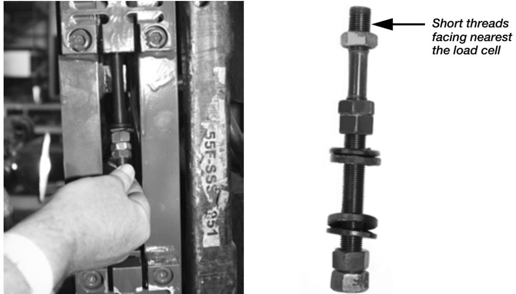
*Figure 2-8. Installing Flexure into Scale*
