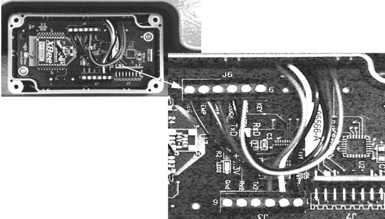
Figure 3-6. Inside of Junction Box - Top Board
