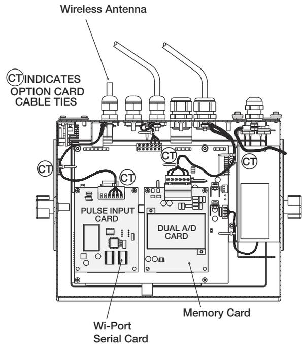
Installed Showing Secured Cables
