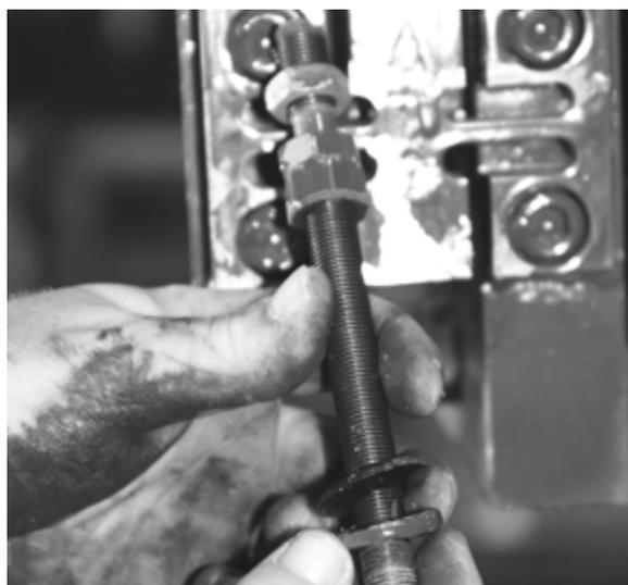
*Ensure flexure rod threads are free of debris and paint by running a nut the full distance of the rod.*
