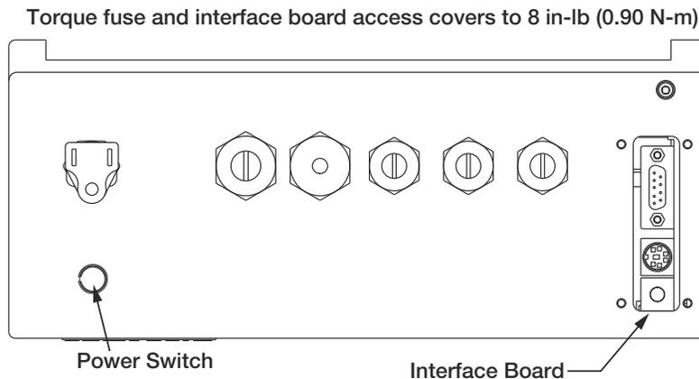
Figure 5-9. Interface Board and Fuse Locations, Universal Model
