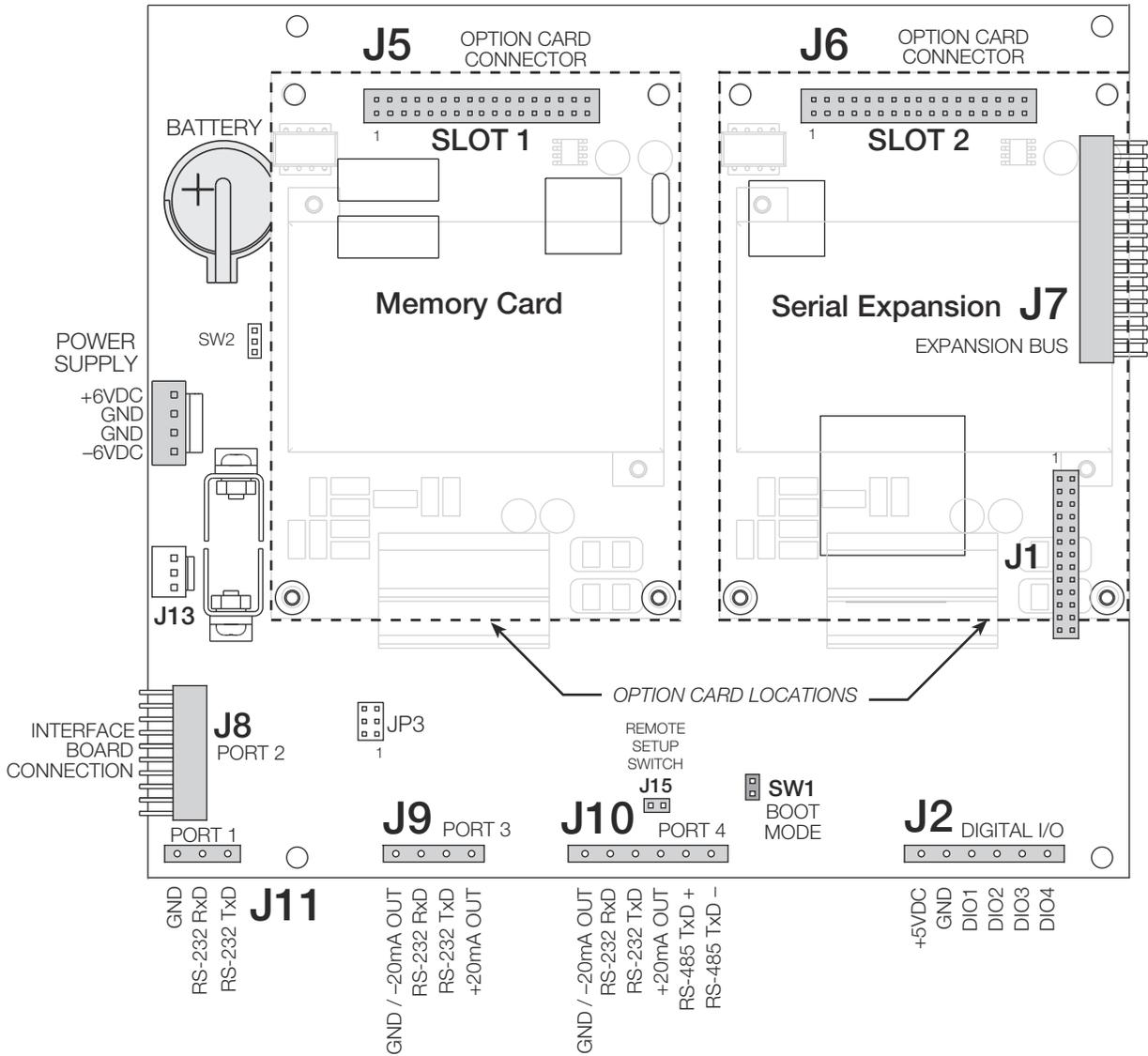
Figure 5-6. 920i CPU Board, Showing Option Card Locations
