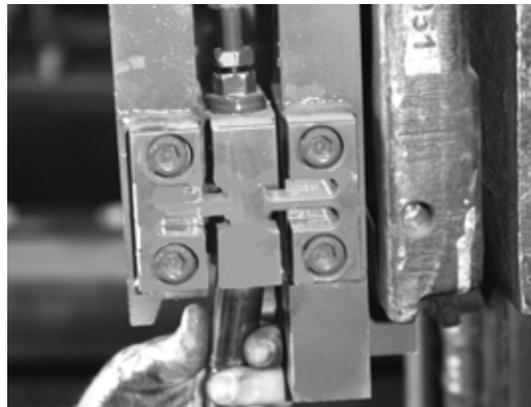
Figure 2-13. Tightening the Lower Hex Nut
