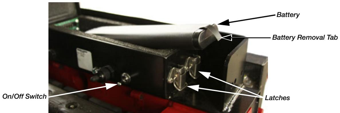
Figure 4-5. Battery Removal and Installation
