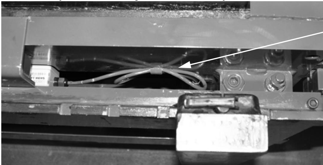
*Detach load cell clip away from back plate of scale using a large screwdriver.*
