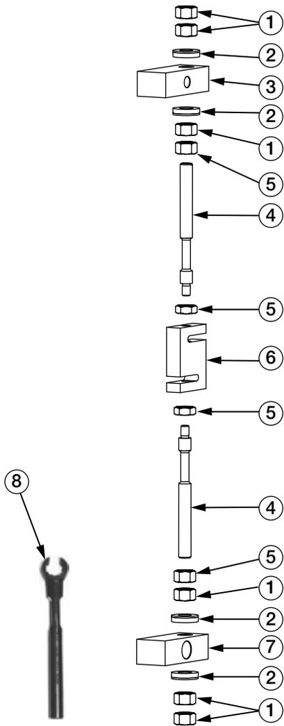
Figure 6-2. Load Cell Replacement Kit Parts Illustration
