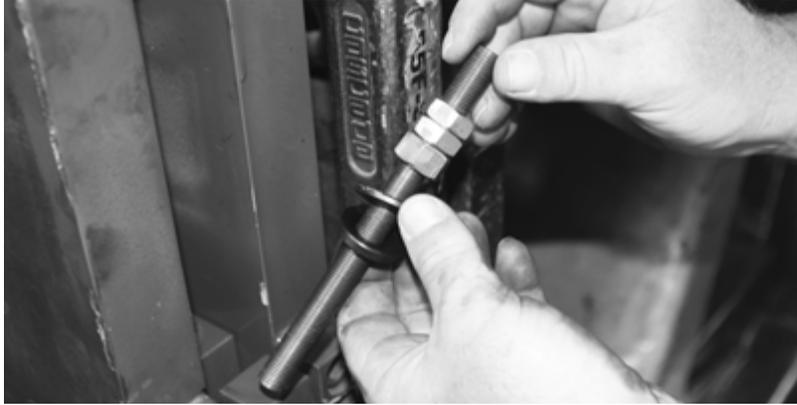
*Figure 2-10. Install Spherical Washer Set*
