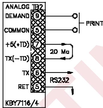
The serial data from the host is provided as a simplex output with the same format as the host.
