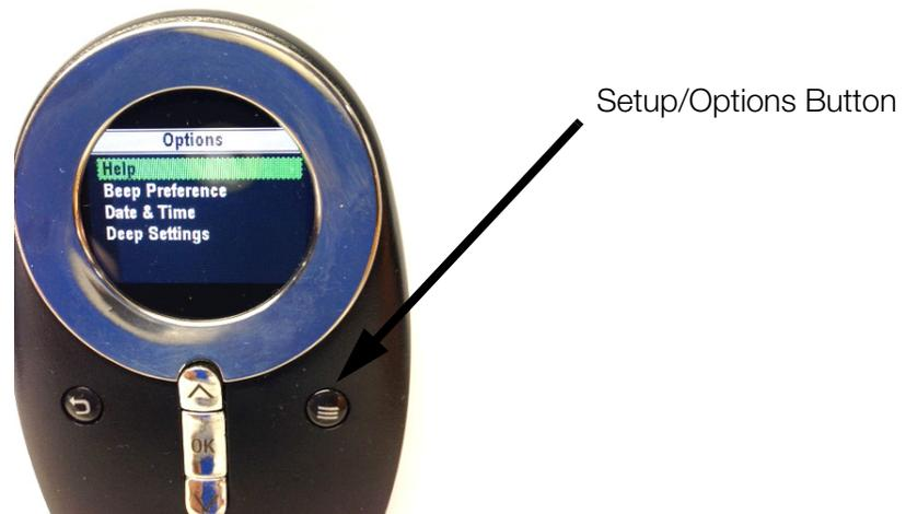
Figure 4-3. Setup/Options Button Location
