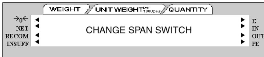
3. While pressing the **REZERO** key, enter 8715 from the numeric keypad to enter the calibration mode.
