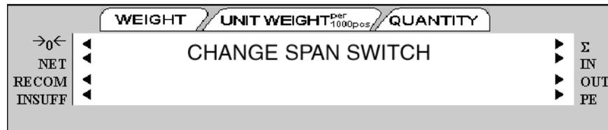
12. Once the span switch is turned off, the scale automatically returns to operation mode. The scale should now be powered off and restarted for the new settings to take effect.
