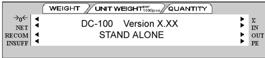
2. After a test of the different elements of the display, the scale takes you to the stand-by screen in the Operation Mode. At the stand-by screen the *WEIGHT*, *UNIT WEIGHT* and *QUANTITY* displays show zeroes and the annunciator for the platform you are using is illuminated (A, B, C or D).
