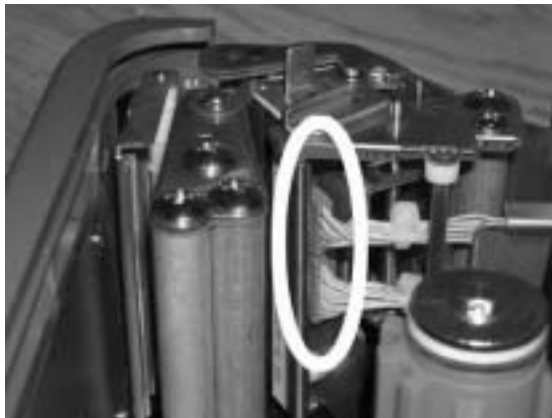
Figure 4-17. Disconnect Printer Cables
