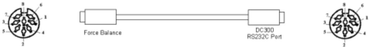
Figure 7-2. Connection from Scale to Force Balance
