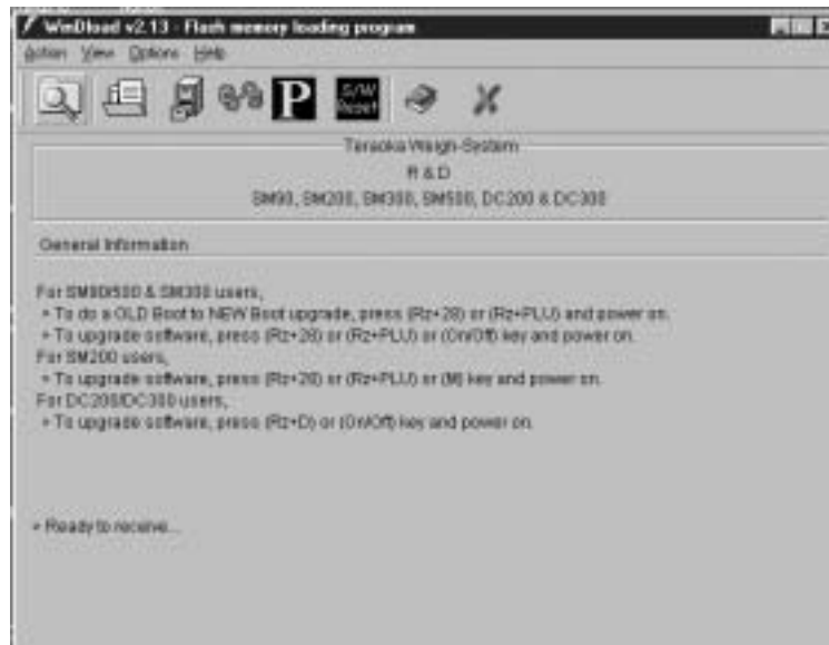
Figure 8-15. WinDload Ready to Receive
