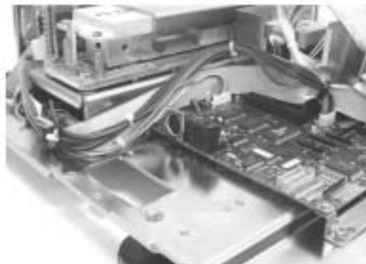
Figure 4-12. Removing the Interface Main Board
