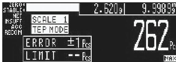
Remove pieces from the platter until you are at or below the maximum safety quantity again. When the scale is stable, the Limit field on the display will reset back to the maximum safe quantity and the characters will change back to white.
