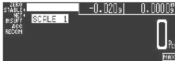
4. To clear the tare weight, press the **TARE** key. The Net indicator lamp will no longer be illuminated.
