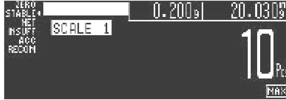
4. To improve the accuracy of the Unit Weight calculation, add another sample of the same pieces. This second sample should be of a number of pieces equal to or fewer than the first one. Press the **PCS** key.
