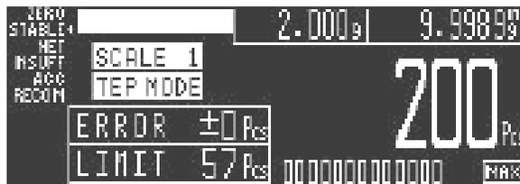
Add pieces up until the quantity limit is reached, then remove the parts from the platter and begin counting again.
