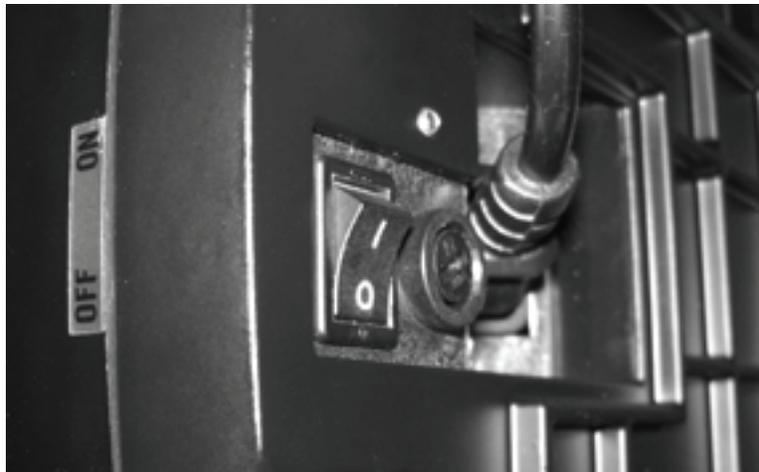
Figure 2-2. AC Plug-in and ON/OFF Switch Location on Underside of DC-530
