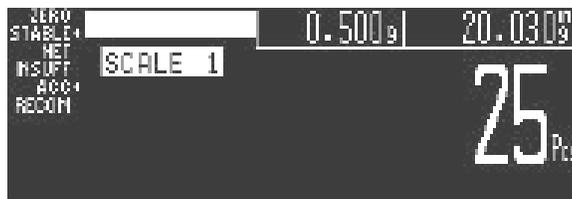
4. Remove Container 1 and place Container 2 (full of parts) on the scale.
