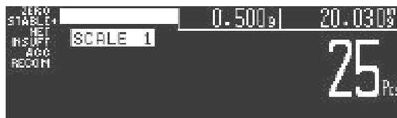
3. Press the **+ (Plus)** key to store the total in Container 1. The Acc (Accumulation) indicator lamp will now be illuminated. The display will show the total quantity of pieces accumulated for 3 seconds, then return to the Counting Mode screen.
