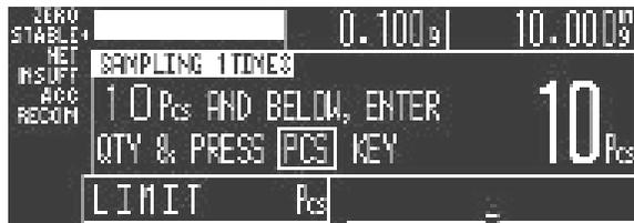
5. To improve the accuracy of the Unit Weight calculation, add another sample of the same pieces according to the number indicated on the display (10 Pcs and below in the example above). Press the **PCS** key. (If the Auto-Recomputing SPEC is set to *1: Auto*, the scale will automatically begin recomputing.)
