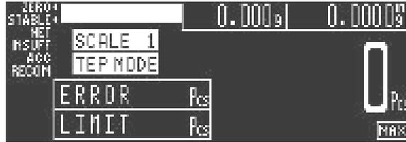
3. Count out a number of parts to be sampled and place them on the scale (for example 10 pieces). For maximum accuracy, count the 10 piece sample into your hand and then add the entire sample to the bin at one time, instead of adding them one or two at a time.
