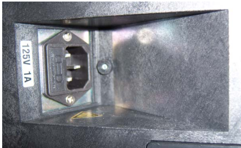
Figure 2-2. AC Plug-in Location on Underside of DC-782
