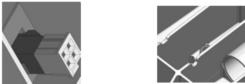
Figure 2-10. Connect Load Cell Cable and Indicator Cable
