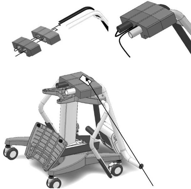
Figure 2-7. Remove Styrofoam Packing Pieces From Main Handle
