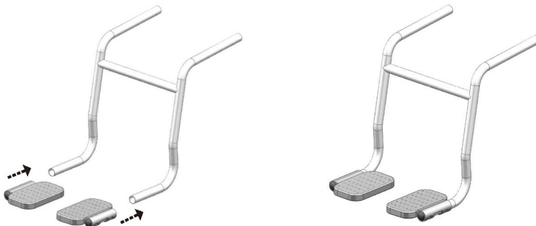
Figure 2-2. Slide and Secure Foot Pads onto Footrest Frame
