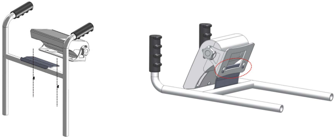
Figure 2-4. Attach Indicator to Handle Assembly
