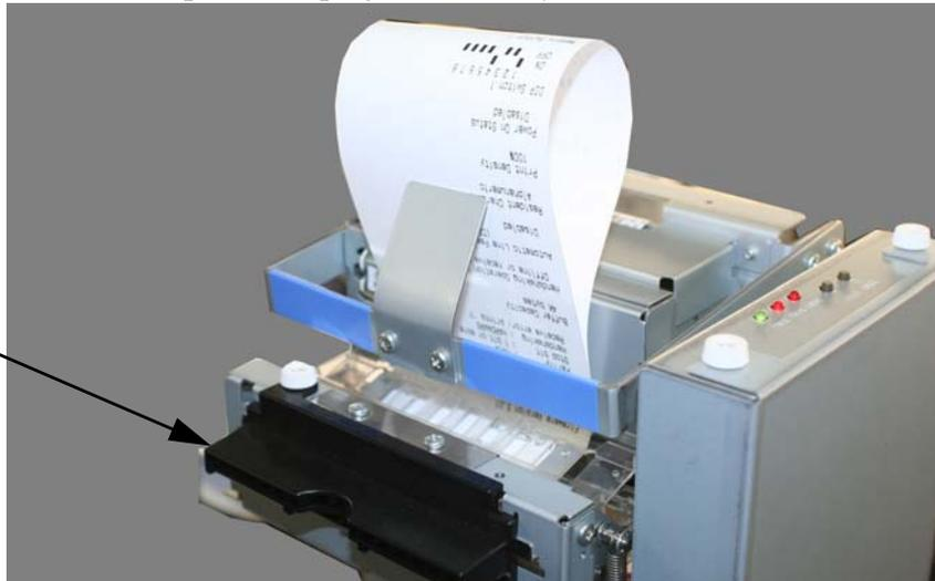
Figure 1. Example of Paper Jamming
