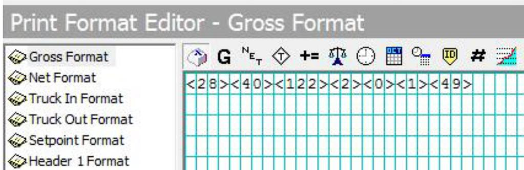
Figure 2. Serial String to Disable the Loop Function
