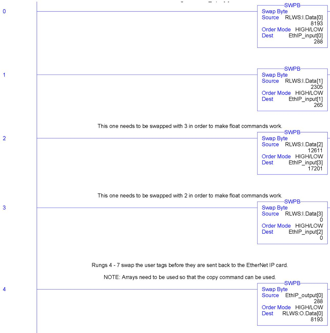
Figure 3-4. Ladder Logic for EtherNet/IP Page 1
