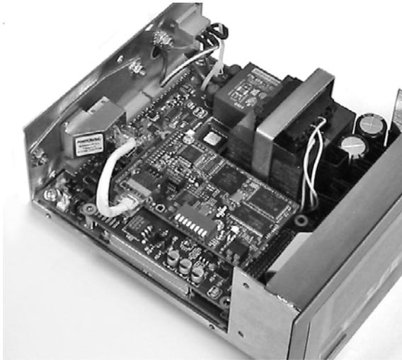
Figure 2-6. EtherNet/IP 520 Backplate Cable Assembly
