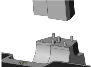
Figure 2-2. Insert Bottom Pillar to Scale Platform
