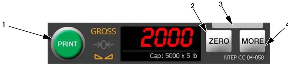
Figure 3-12. VIRTUi2 Operator Mode
