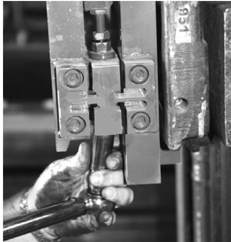
*Figure 6-13. Tightening the Lower Hex Nut*
