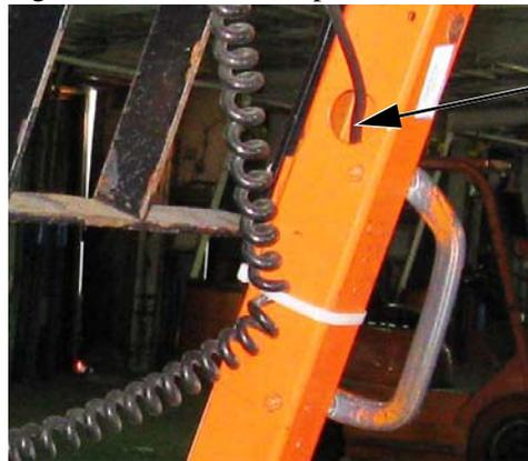
Run power cable through chassis to forklift battery.
