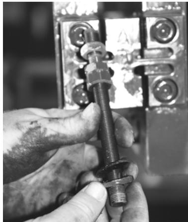
Ensure flexure rod threads are free of debris and paint by running a nut the full distance of the rod.
