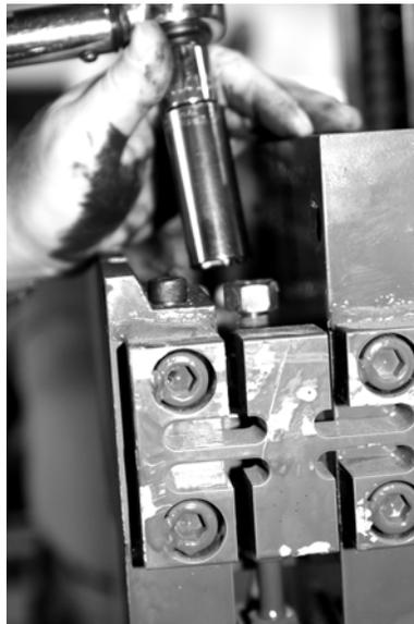
*Figure 6-3. Removal of Hex Nut (#1 of Parts Breakdown)*
