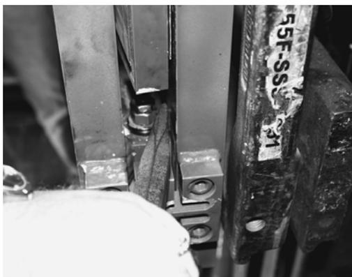
*Figure 6-12. Centering the Load Cell Using a Chisel*
