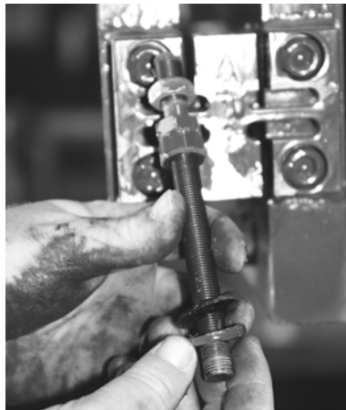
Figure 6-5. Remove Flexure Rod with Nuts and Washers
