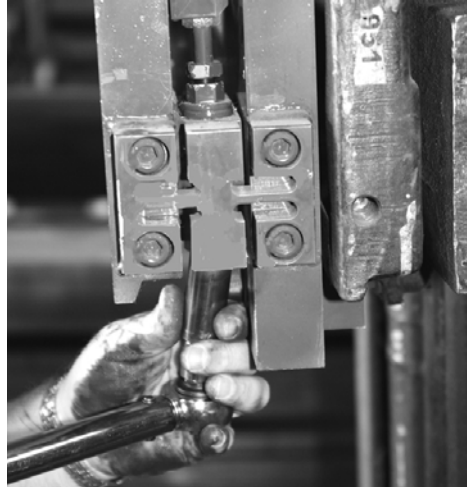
Figure 6-13. Tightening the Lower Hex Nut
