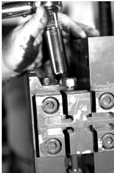
Figure 6-3. Removal of Hex Nut (#1 of Parts Breakdown)
