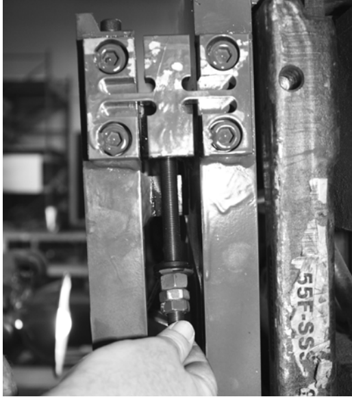
Figure 6-8. Installing Flexure into Scale
