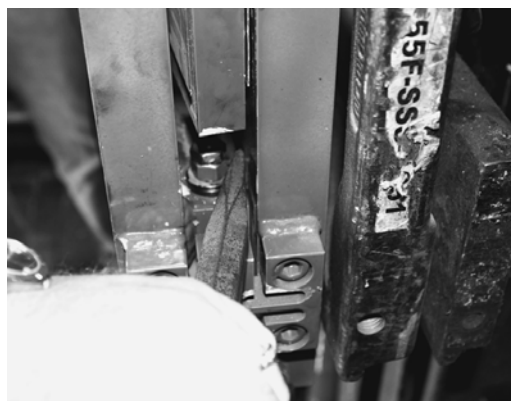
Figure 6-12. Centering the Load Cell Using a Chisel
