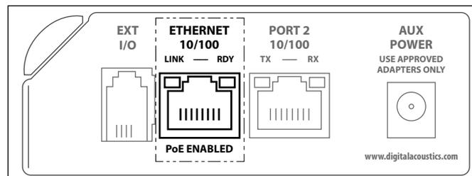
Figure 2-6. IP Endpoint Amplifier Ports
