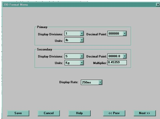
Figure 3-1. Sample Revolution Format Display
