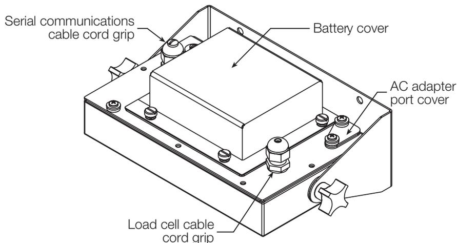
Figure 2-1. 390-DC Backplate, Showing Key Component Locations
