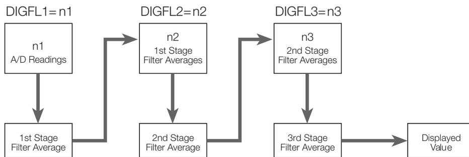
Figure 8-4. Flow Diagram for 390-DC Digital Filters
