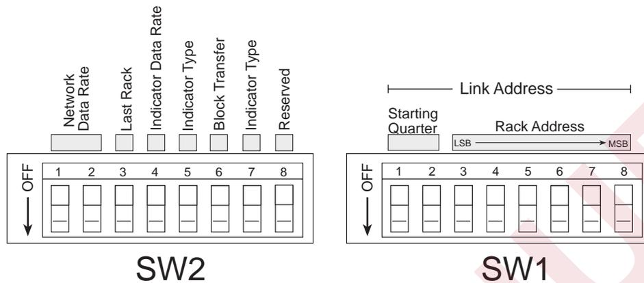
Figure 2-8. SW1 and SW2 DIP Switch Assignments
