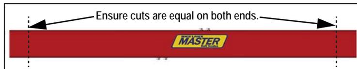
Figure 2-7. Resize Weighframe – 311M Only
