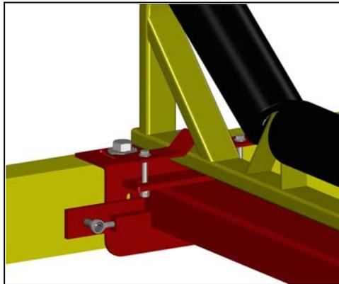
Figure 2-11. Transport Lockout
