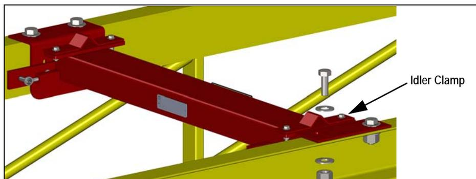
Figure 2-9. Installed 711 Weighframe
