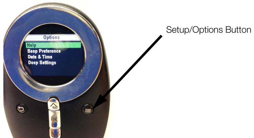
Figure 4-3. Setup/Options Button Location
