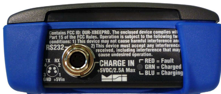
Figure 2-1. Battery Charger Plug-In
