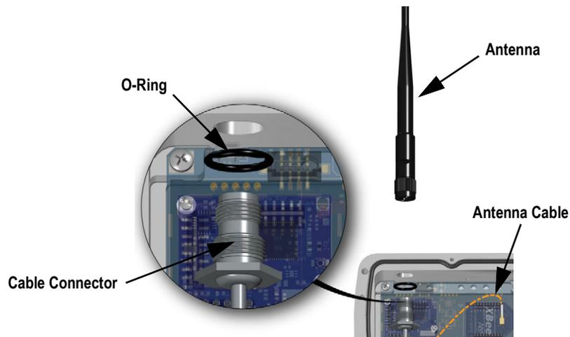
Figure 2-8. Replace Antenna
