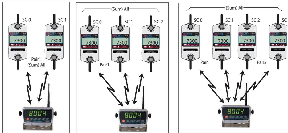
Figure 6-1. Multiple Sensor Network
