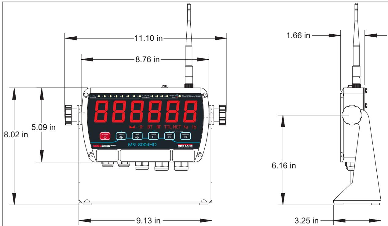
Figure 8-1. Mechanical Dimensions
