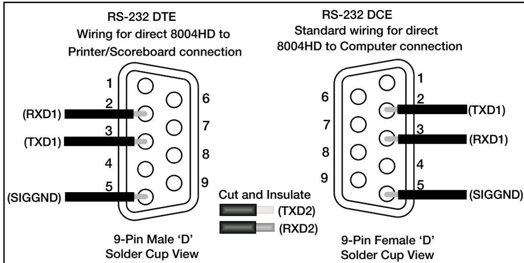
Figure 6-4. Communication Wiring
