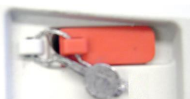
Locked with Wire Seal
