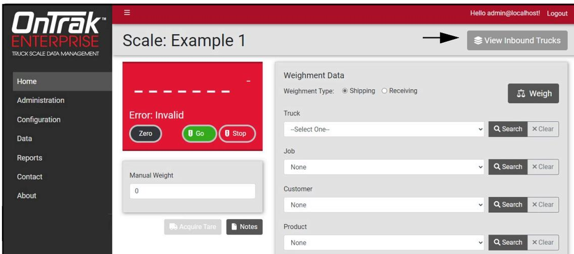
Figure 9-19. Scale page with View Inbound Trucks Identified
