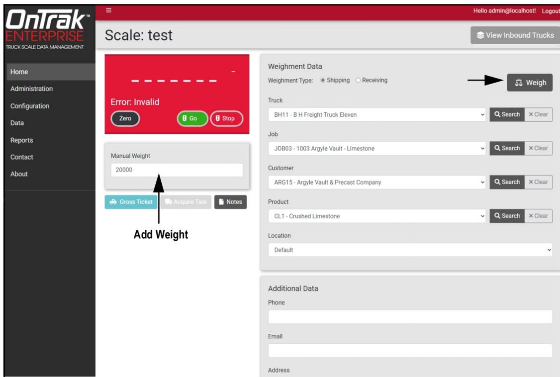
Figure 9-25. Scale page with Manual Weigh Field
