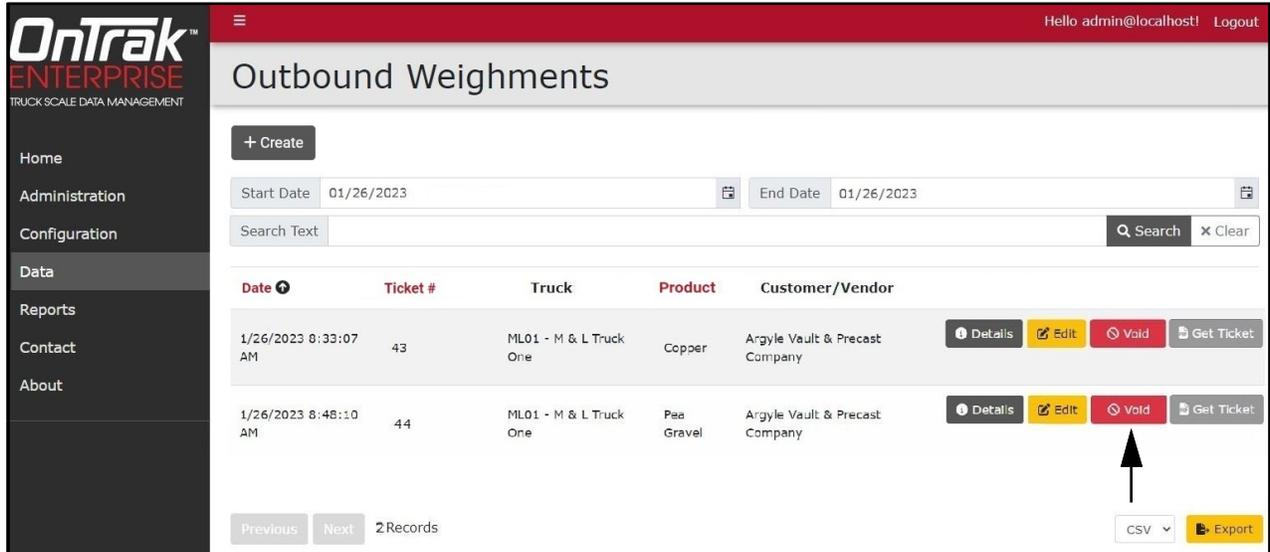
Figure 7-42. Outbound Weighments Page with Void Button Identified
