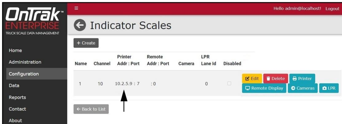
Figure 6-10. Indicator Scales Page with Printer Information
