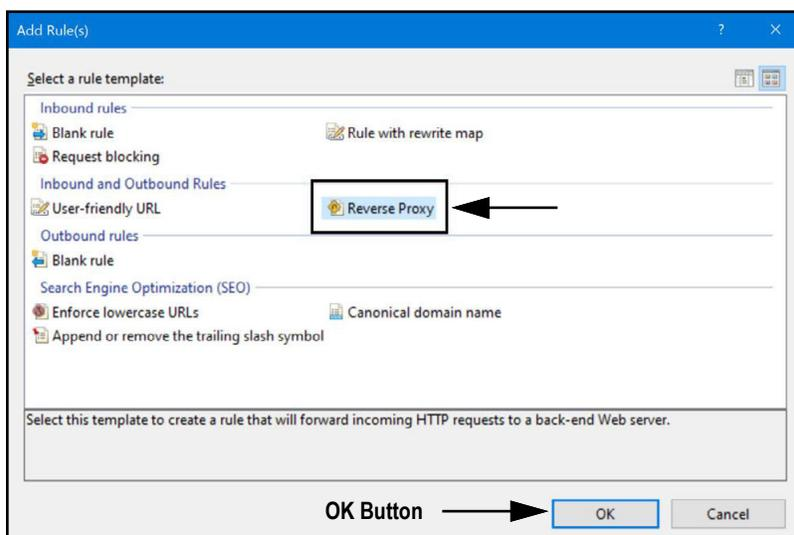
Figure 2-10. Add Rules Window with Reverse Proxy Identified
