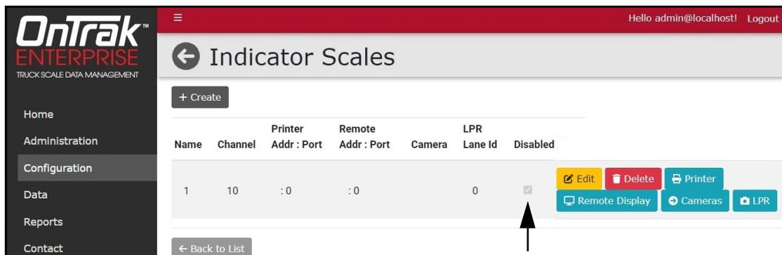
Figure 6-26. Indicator Scale Page with Scale Disabled
