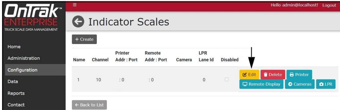
Figure 6-24. Indicator Scale Page with the Edit Identified
