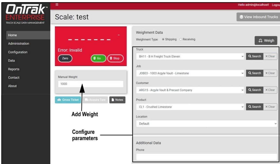
Figure 9-16. Scale page with Manual Weight Field
