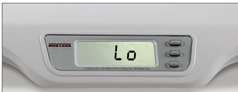
Figure 2-2. Low Battery Indicator
