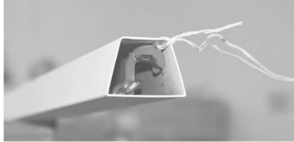
Figure 2-6. Remove Twist Tie from Steelyard Rod
