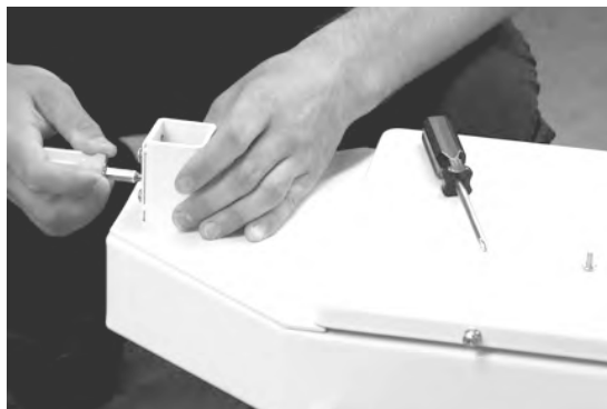
Figure 2-5. Remove Screws from Scale Base
