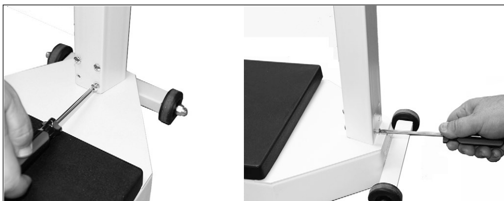
Figure 2-4. Secure Pillar to Scale Base
