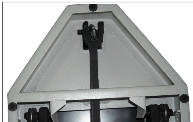
Figure 2-7. Steelyard Rod Connected
