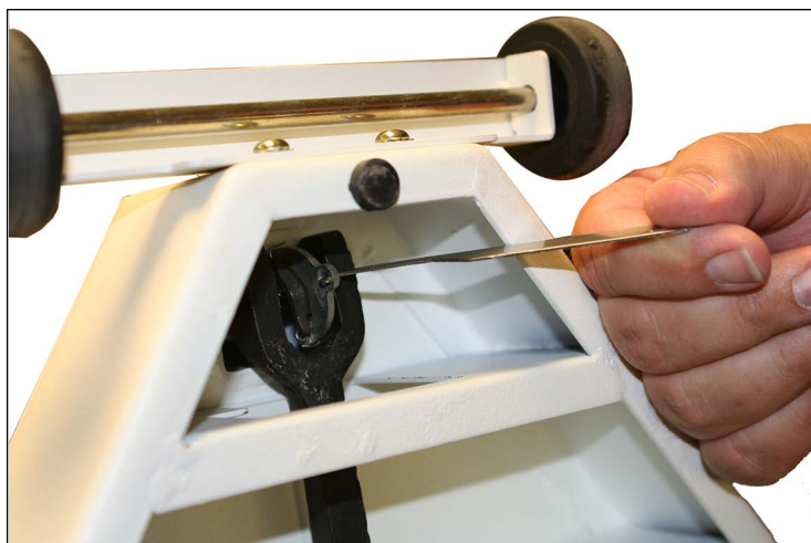
Figure 2-6. Connect Steelyard Rod to Scale Base
