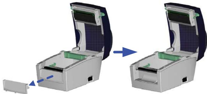
5. Push the cutter connector into the printer through the cable hole as shown in the figure to the right.
