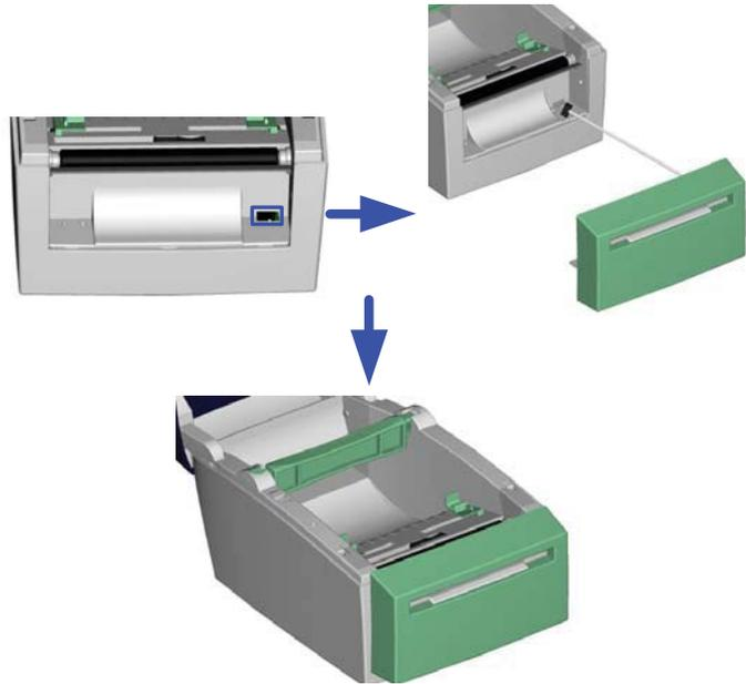
7. Turn the printer around and tighten screws to secure the cutter module.
