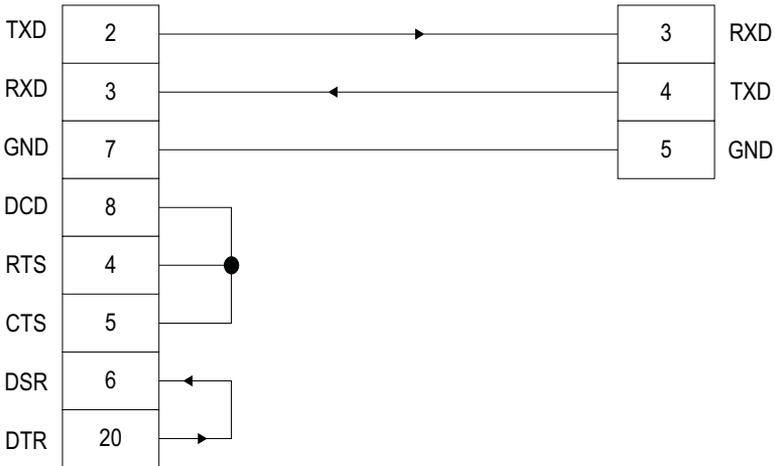
Figure 2-8. Sample connection with PC9801
