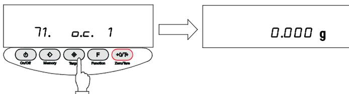
Figure 2-5. Terminating the Function Selection
