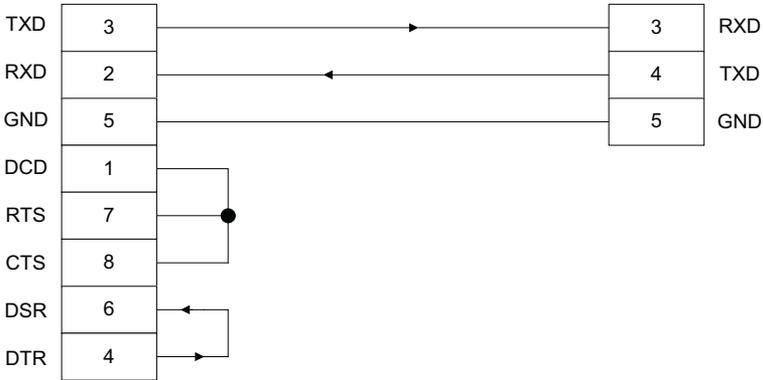
Figure 2-7. Sample connection with an IBM-PC/AT compatible
