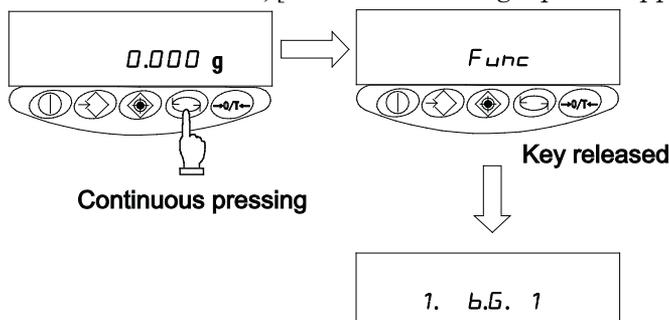
Figure 2-1. Invoking the Function
