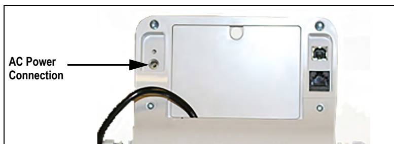
Figure 2-10. Power Connection Site
