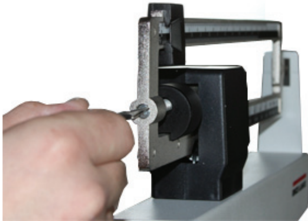
Figure 4-2. Zero Adjusting Screw Location
