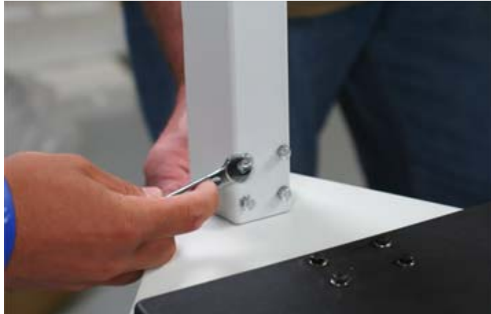
Figure 2-4. Attach Eight Bolts and Washers to Secure the Pillar to the Scale Base
