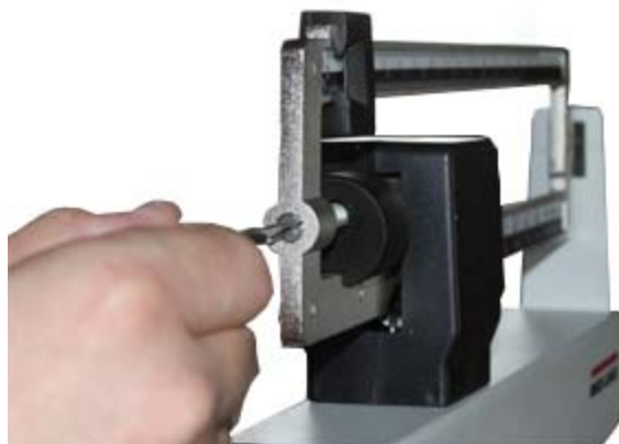
Figure 4-2. Zero Adjusting Screw Location
