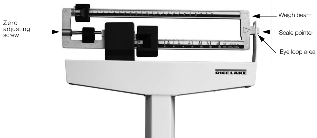
Figure 3-1. Eye Loop Area and Zero Adjusting Screw Location (Lb and kg version without height rod shown)
