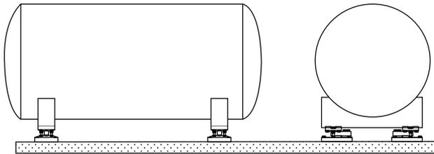
Horizontal tank with four point support. Weigh modules oriented with exiting toward pairs on each end.
