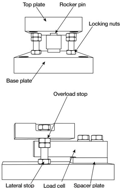
Figure 2-3 Lateral and Overlift/Overload Stops
