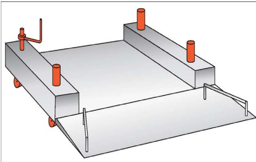
4 built-in foldaway wheels which can be lowered for easy handling of platform
