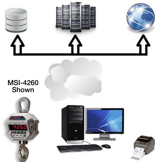
Figure 1-1. Quick Start - Connecting to the Network
