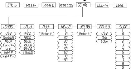
Figure 2-3. Serial Communications Menu Structure
