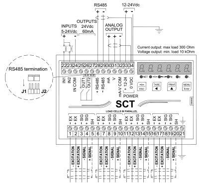
2 outputs: configurable setpoints or remote output management via protocol.
