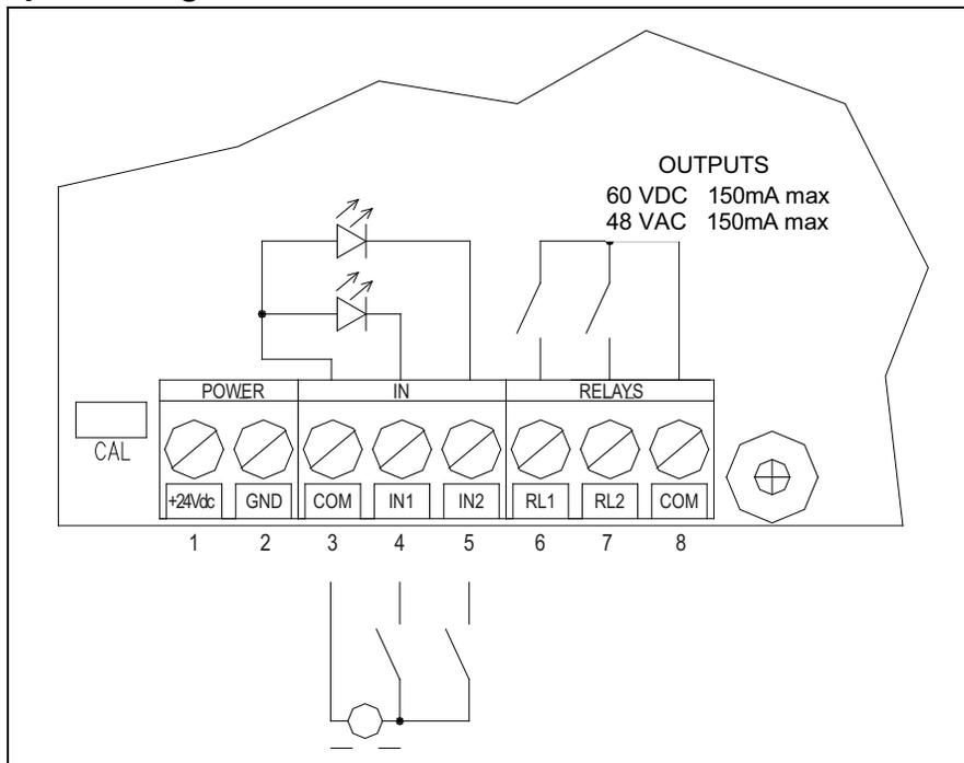
Figure 2-5. Input/Output Wiring
