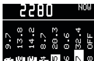
Figure 2-3. Current Load Distribution Display
