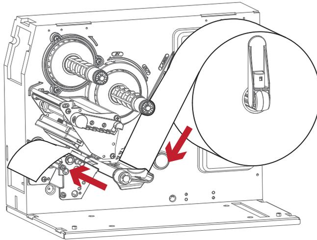
5. Pass the label stock through the adjustable sensor and up to the tear-off plate.
