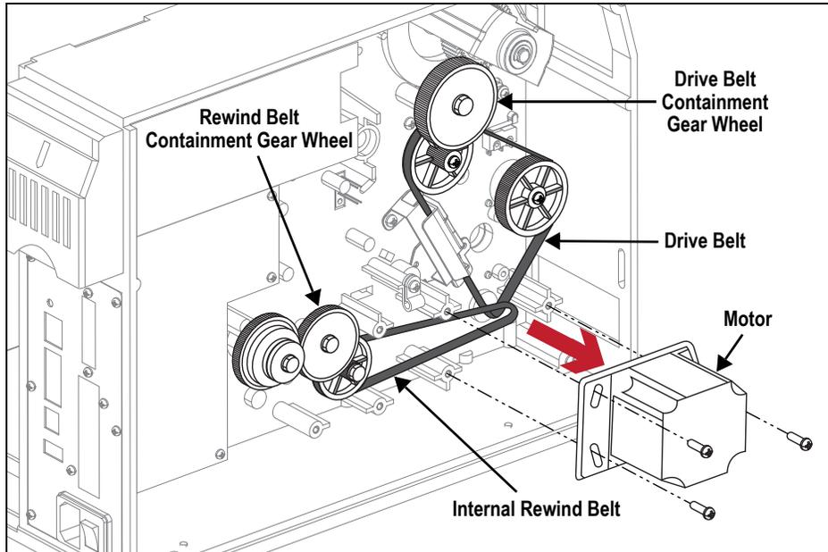
3. Remove the belt containment gear wheel, of the belt being replaced, using a 10 mm socket or wrench.
