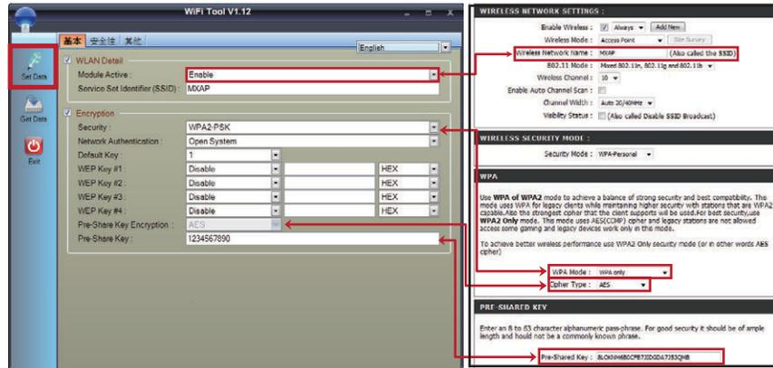
2. Click **Set Data** button after the parameters are completely set. Approximately 5 seconds later, the printer will automatically reboot.
