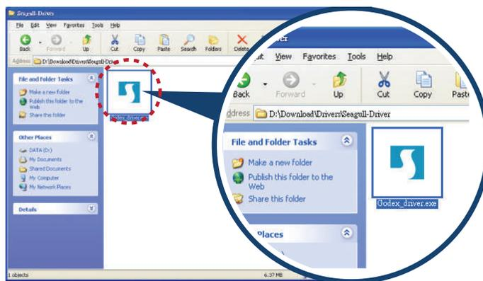
2. Follow the instructions on the screen. The Driver Wizard guides through the installation procedure. Select **Install printer drivers**.
