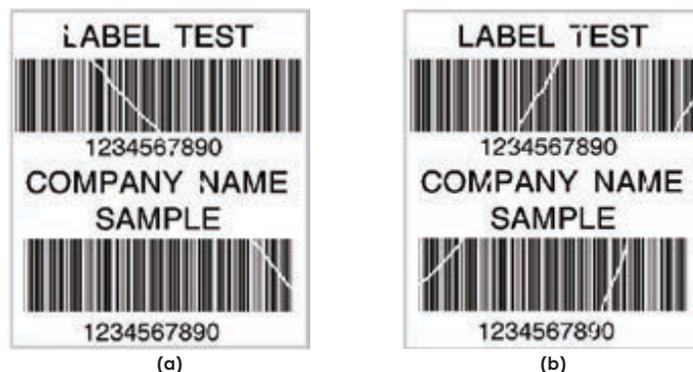
To keep track of the change in print quality, adjust the screws by half a turn at a time. Print a test page. If there is no improvement in the print result, turn the screw by another half turn. Do not turn the adjustment screw more than two full turns (360°).
