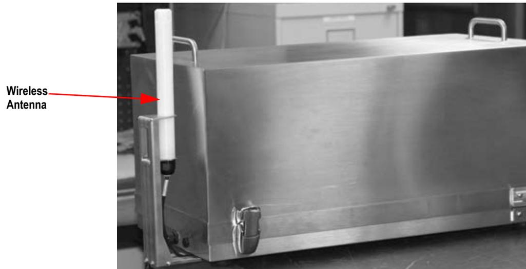
Figure 5-35. Installed Wireless Antenna
