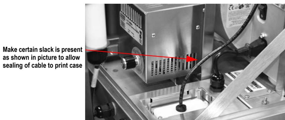
Figure 5-33. Keep Proper Amount of Slack in Cable
