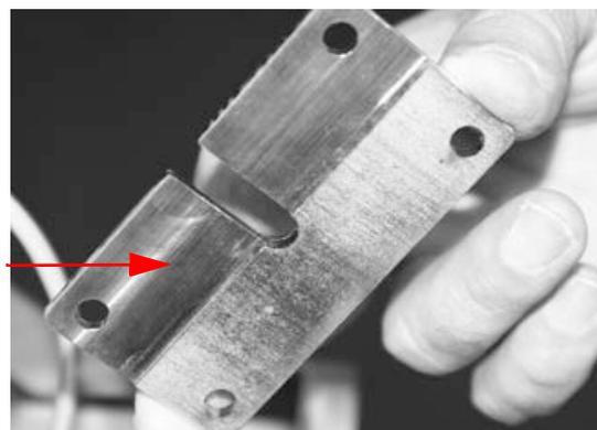
Clamp plate - note the step for the half plate
