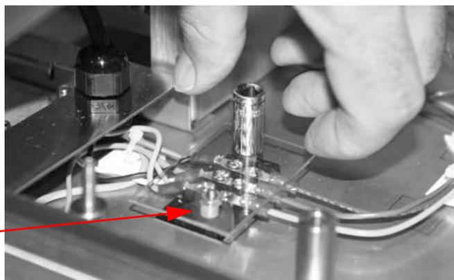
Figure 5-13. Replace Clear Plastic Cover and Gently Tighten
