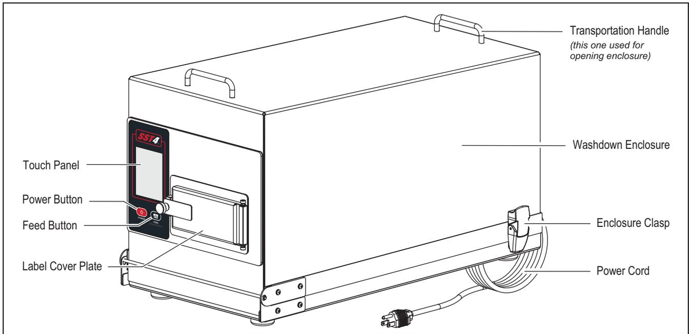
Figure 1-1. Printer Front View
