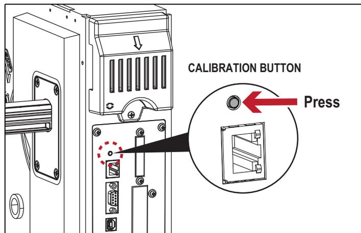
Press Calibration button for 2 seconds, it uses auto-sensing to calibrate the label and ribbon's parameters.
