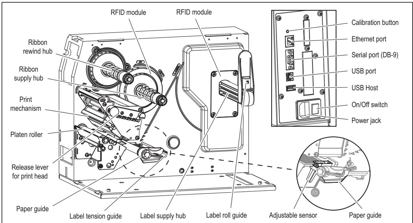
Figure 1-2. Printer Internal Views
