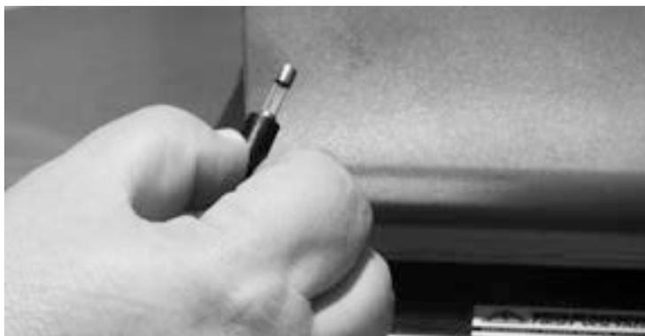
Figure 5-19. Remove Actual Fuse From the Receptacle and Replace with a New Fuse
