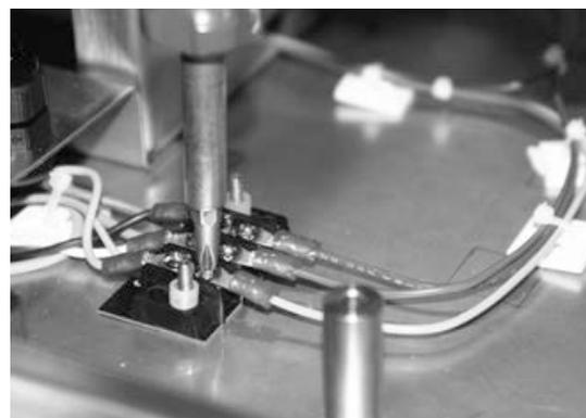
Figure 5-12. Connect Wiring Harness to Terminal Strip
