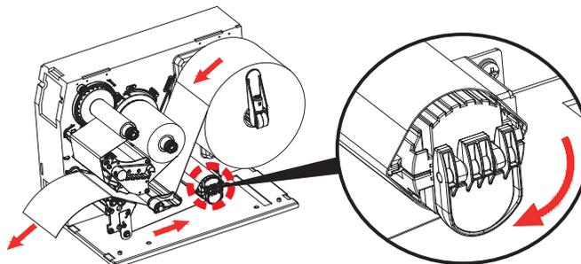
3. Pull the liner back to rewinder shaft and rotate it 2~3 circles.
