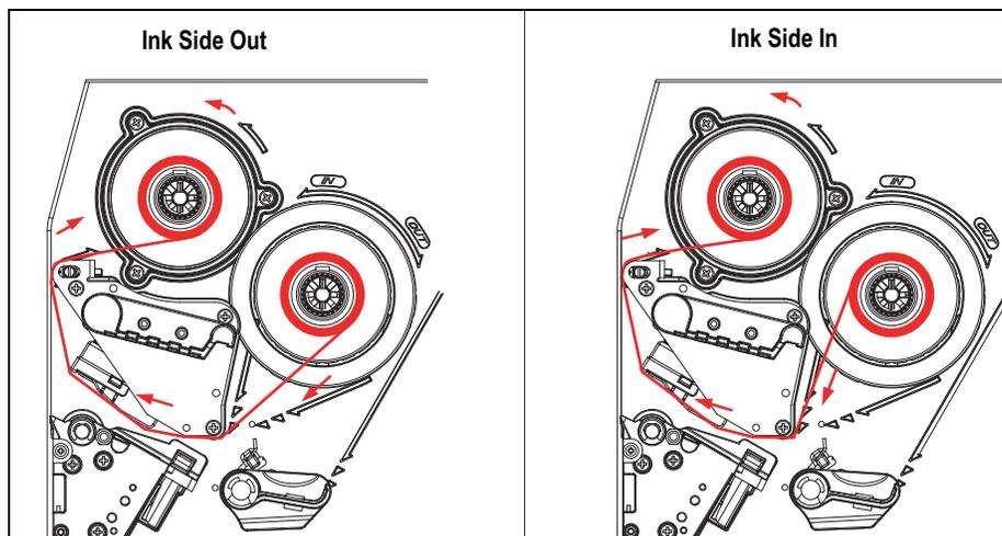
3. Pass the ribbon under the printhead and back up on the other side. Attach it to the empty ribbon core on the ribbon rewind hub.
