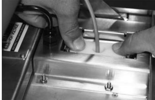
Figure 5-29. Seat the Split Seal Assembly
