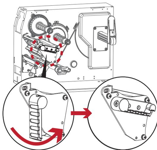
3. If no improvement is visible, turn the screws clockwise or counterclockwise as far as possible and be sure to align with the indicator board and indicator line. Repeat the adjustment process until printing quality has improved.
