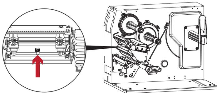
2. Turn the printhead release lever counterclockwise to the top right position.
