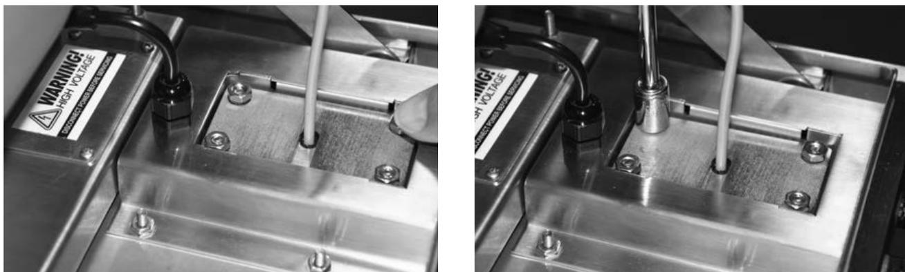
Figure 5-32. Tighten Up The Entire Assembly
