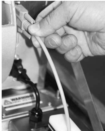
Figure 2-9. Connect Communications Cable to Back of Printer
