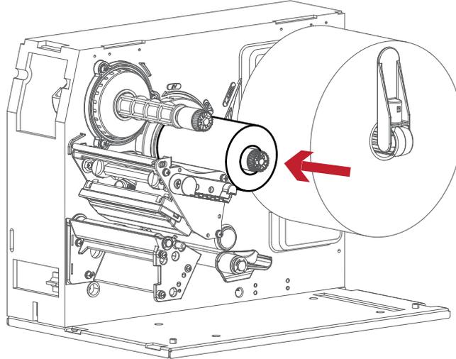
2. The two illustrations below show how to install the ribbon depending on the ribbon type (ink side in or out).
