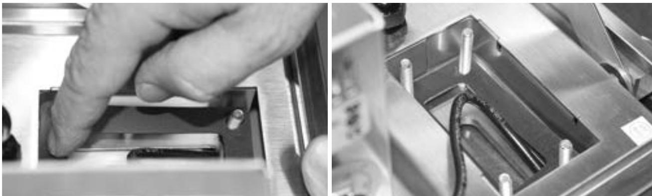
Figure 5-26. Press Down Rubber Gasket Around Bolts
