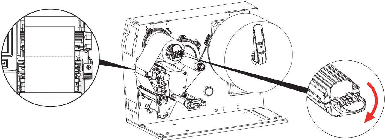
2. Pull open the knob, ribbon could be easy to remove.
