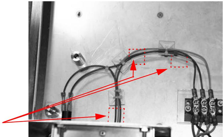
Figure 5-14. Secure Square Adhesive Cable Ties to SST4 Enclosure Bottom
