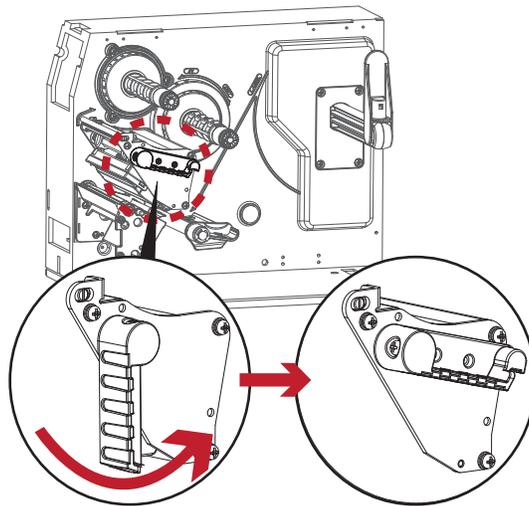
3. Hold the printhead module, pull out the TPH cable smoothly.
