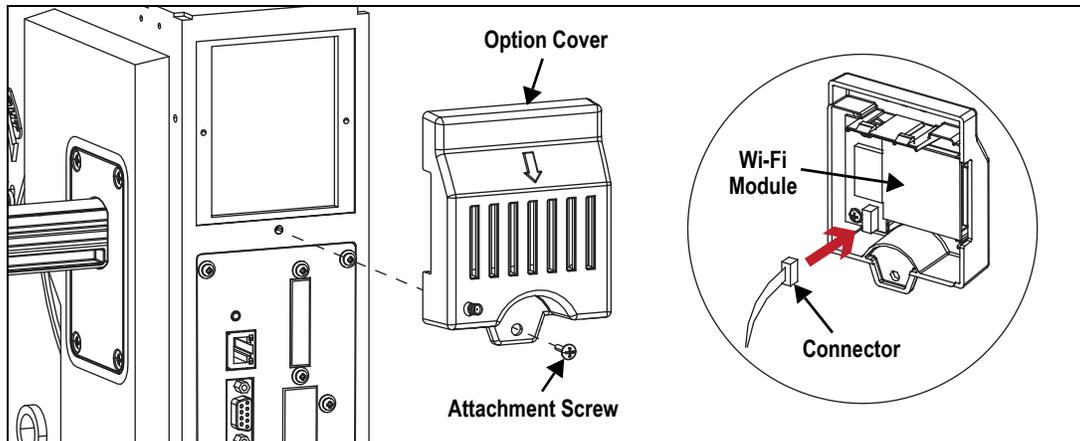
3. Remove the option cover and disconnect the connector.
