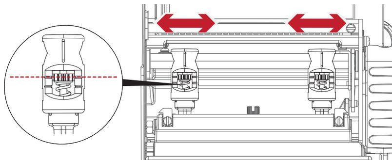
3. Turning the screw left increases the pressure, while turning it right reduces the pressure. Mark (B), be sure not to turn the screw so that it goes below Mark (B).
