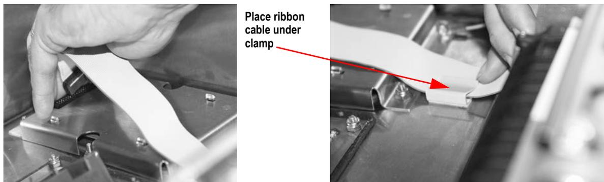
Figure 5-17. Re-Attach Ribbon Cable
