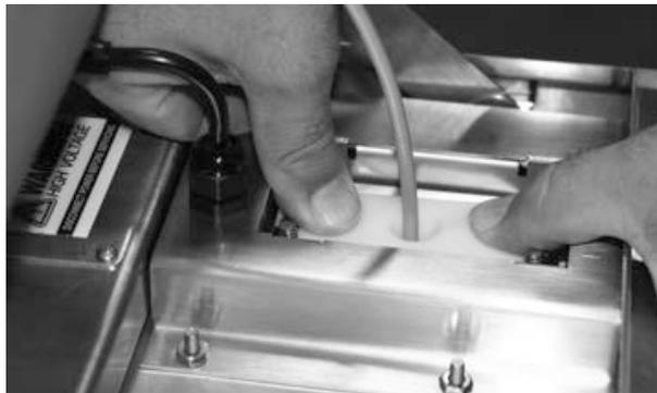
Figure 2-10. Seat the Split Seal Assembly
