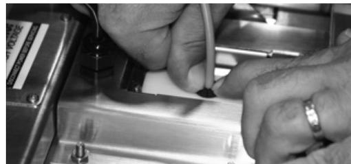
Make certain slack is present as shown in picture to allow sealing of cable to print case
