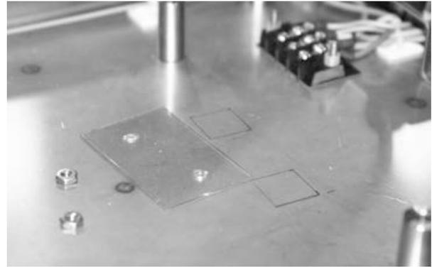
Figure 5-8. Terminal Strip Location, Wiring, and Clear Cover
