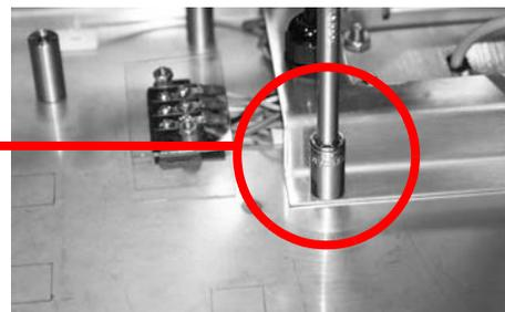
Figure 5-10. Secure Heater to Enclosure Bottom
