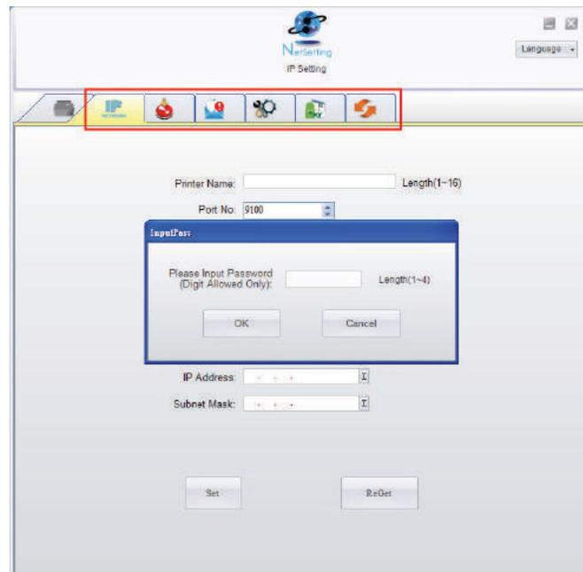
There are six tabs at the top of the interface window which can configure different types of network settings. The correct password is needed to enter the configuration pages for data security.
