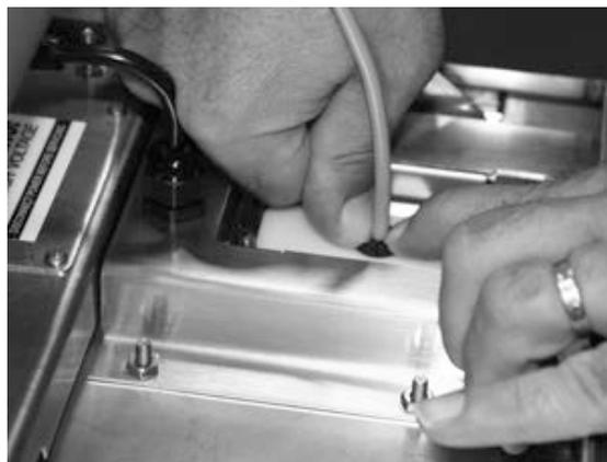
Figure 2-11. Insert Split Grommet Onto the Split Seal Plates
