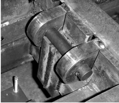
Figure 2-3. Pin and Receptacle Interface
