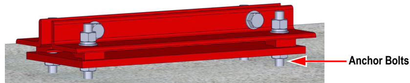
Figure 2-10. Approach Plate on Anchor Bolts
